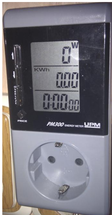
Figure 6. UPM Energy Meter MP300
