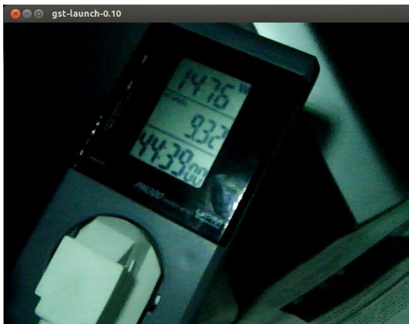
Figure 1. GSTlaunch-0.10 - monitoring system of readings of UPM Energy Meter MP300
