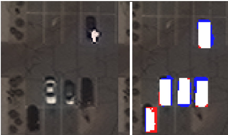
Figure 3.1. Semantic pixel-level segmentation of the “light vehicles” object class in satellite imagery. Input image (left) and output image (right)
